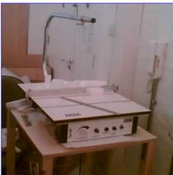
This machine cuts out the shape of the building
